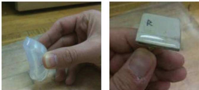
Figure 1b. Biocompatibility issues for implantable patch antennas: thin-layer encapsulation [20].
