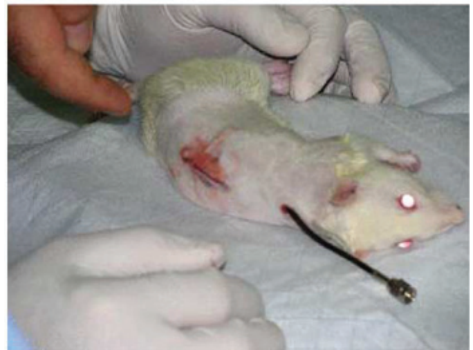
Figure 9b. The testing of an implantable patch antenna inside animal tissue: a antenna surgically implanted into a rat [20].
